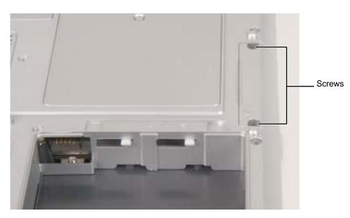
**5** Remove the hard drive kit screws.
