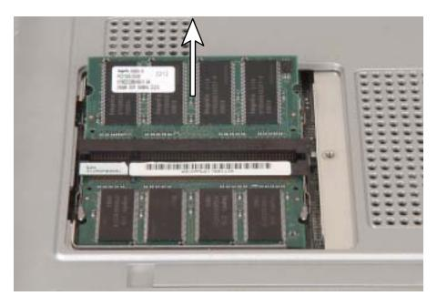
**7** Pull the memory module out of the slot.
